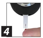
With Test Strip still in Meter, touch Sample Tip to top of blood drop and allow blood to be drawn into Test Strip. Remove from blood drop immediately after Meter beeps and dashes appear across Meter Display.
