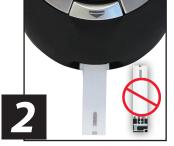
Remove test strip from vial and close vial immediately. Insert Test Strip into Test Port with Contact End (blocks facing up). The Meter turns on.
