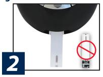
Remove Test Strip from vial and close vial immediately. Insert Test Strip into Test Port with Contact End (blocks facing up). The Meter turns on.
